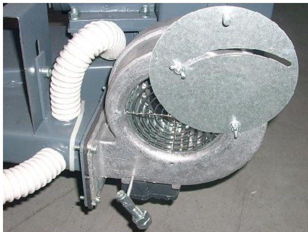
Figure 13. Position max. open of the fan flap
