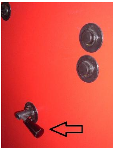
Figure 17. Position of flap handle (working position)
