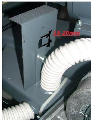
Figure 14. Position of fan flap.
