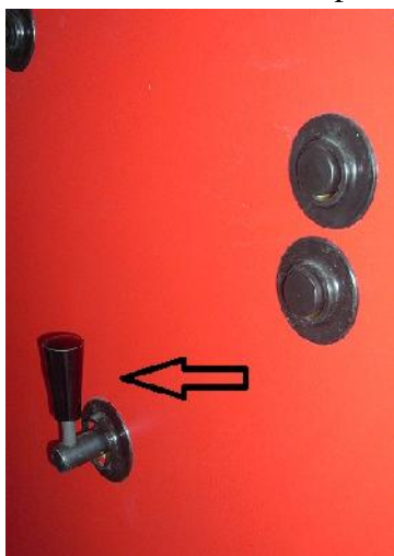
Figure 15. Position of flap handle for- INITIATING FIRE
